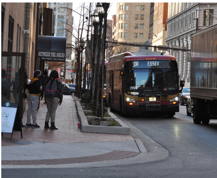
Travelway widths balance narrow lanes for speed control vs. safely accommodating the movement of transit and trucks.
