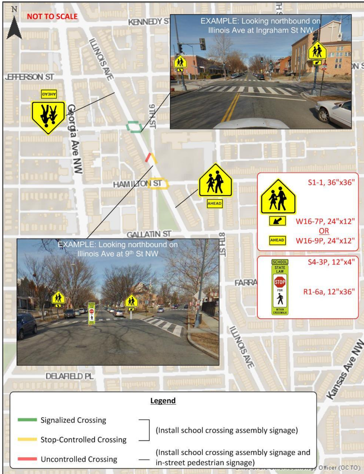
Figure 8: Recommended Improvement – Install School Crossing Assembly Signage
