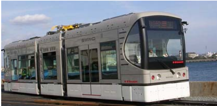
Streetcar SWIMO powered by both overhead lines and nickel metal-hydrate battery
